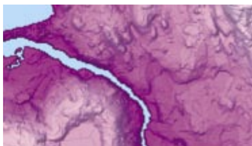
Colour Triangular Irregular Network (TIN) created from Enhanced DTM
